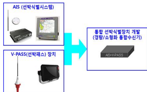
Fig. 4. Small / Light weight integrated ship identification system for aircraft
