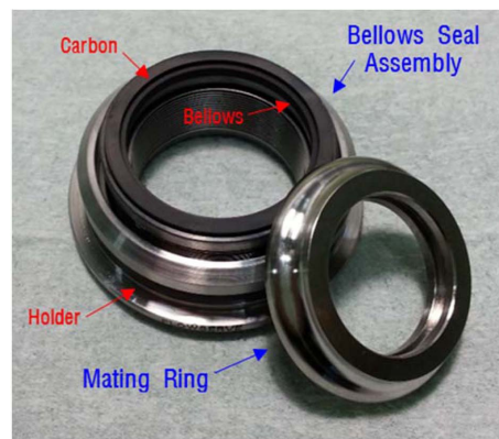
Fig. 3. Prototype of turbopump mechanical face seal.
