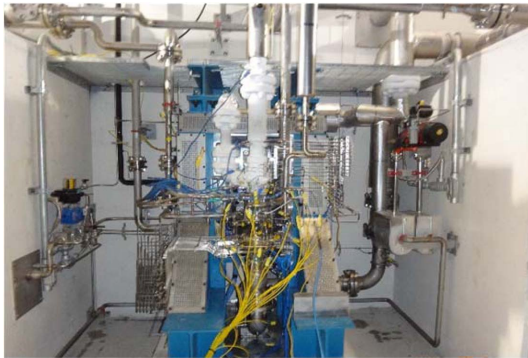
Fig. 8. 7-ton class turbopump real-propellant test.
