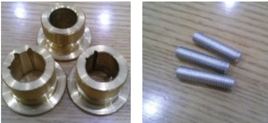
Fig. 8 Bearing and misalignment damage
