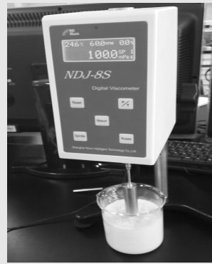
Figure 2. Rotation Viscometer (Shanghai Nirun Intelligent Technology Co.,Ltd. NDJ-8S)
