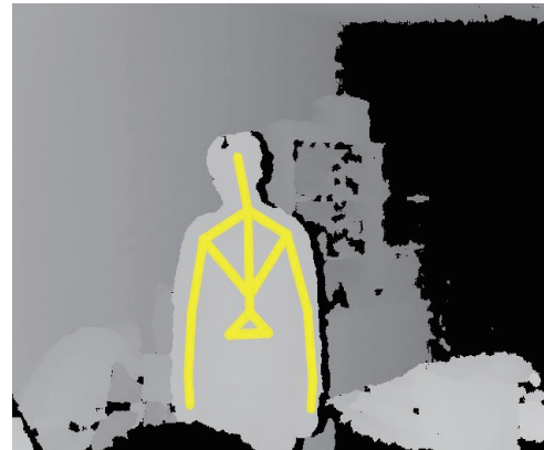
Fig. 2. Depth image and Skeleton Data extraction
