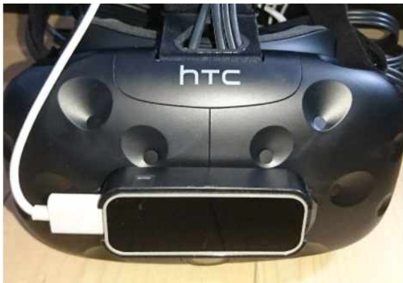
Fig. 3. Leap motion mounted to HTC Vive
