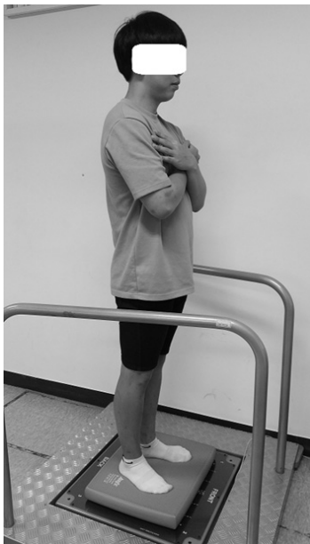
Fig. 1. The experimental posture for LOG measurement on balance training system with unstable support surface.
