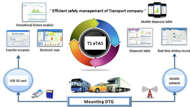
〈Fig. 2〉 Outline of Digital Tachograph Analysis System
