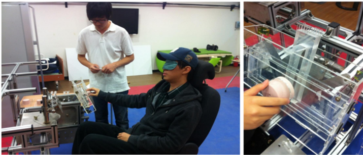
Figure 1. Experimental apparatus and scene with knob height variation
