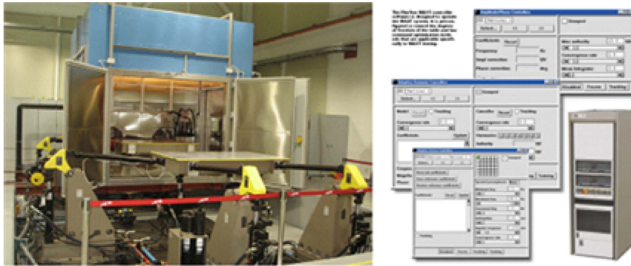
Fig. 7. Photograph of MAST(MTS model 323.40)
