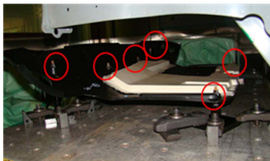
Fig. 8. Photograph showing the check points for torque according to the KLT method
