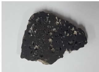
(b) Section of steelmaking slag containing numbers of voids
