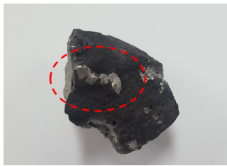
(a) Steel present in the steelmaking slag
