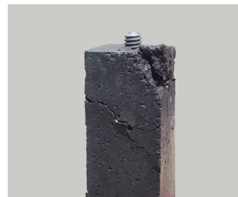
(a) Cracks of specimen
