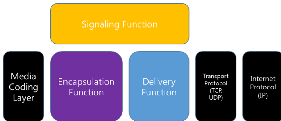
Fig. 2. MMT Layered Structure
