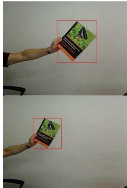
Fig. 2. Result of object detection and tracking with implemented system based on improved Camshift+SURF.
