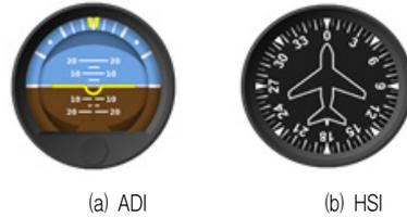
Fig. 6. Flight data panel
