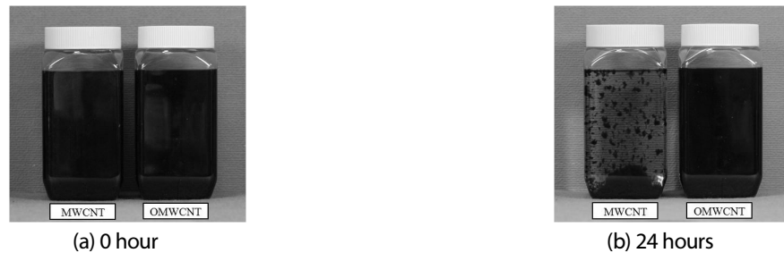
Fig. 4 Comparison of stability of dispersion according to elapsed time after ultrasonic dispersion and oxidation treatment with carbon nanotube nanofluids
