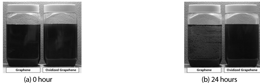
Fig. 5 Comparison of stability of dispersion according to elapsed time after ultrasonic dispersion and oxidation treatment with graphene nanofluids
