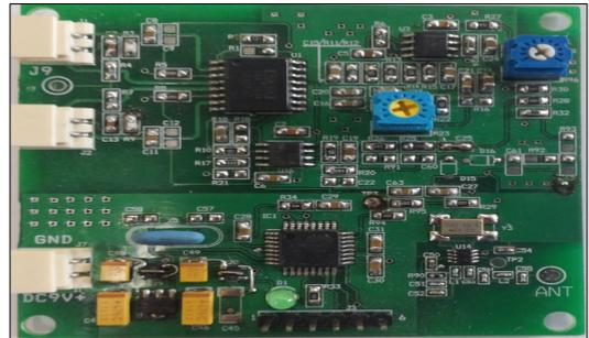
[Fig. 5] PCB of impedance measuring system
