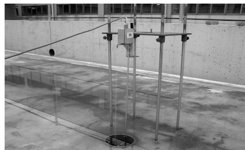
Fig. 5. Installation of wave height meter
