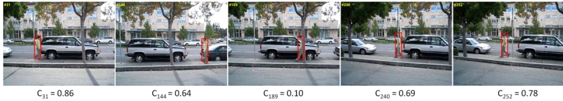
Fig. 2. Examples of the varied confidences. The confidence C_t at frame t is the maximum value of all candidates in the searching region, which is predicted by the proposed AI-ELM tracker.
