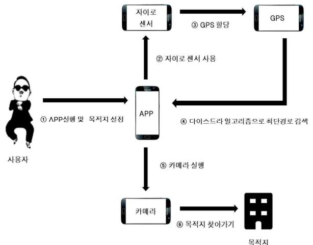
Fig. 5. System Structure
