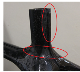
(a) Cracked frame
