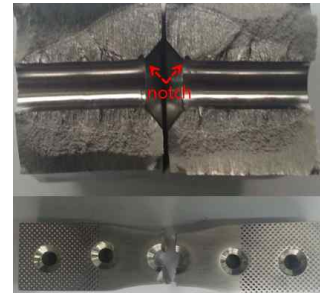
Fig. 12 Fractured FCL W2 specimen
