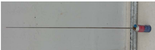
Fig. 10. Torch for use as an ignition device.
