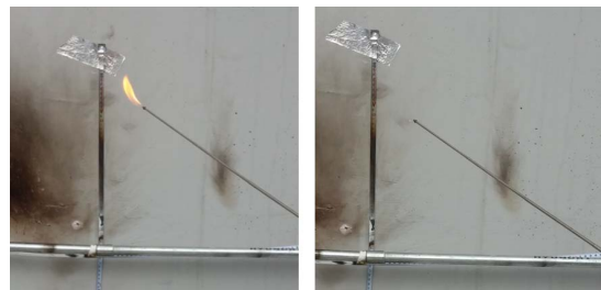
Fig. 11. Flame and fire extinguishing on torch.
