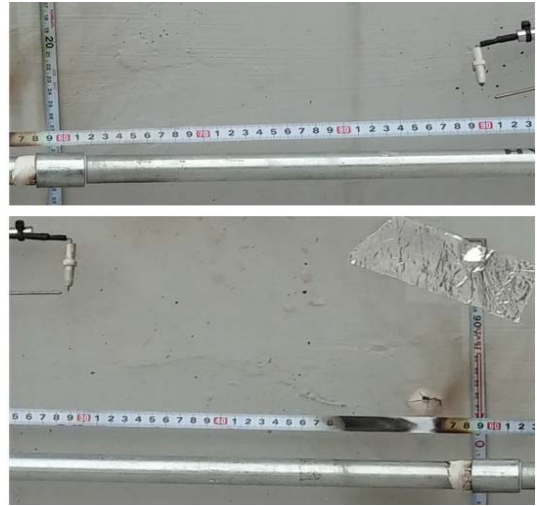
Fig. 8. Igniters located 30 cm right and left upper each.
