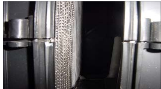
Fig. 5. Inner shape example of evaporator.
