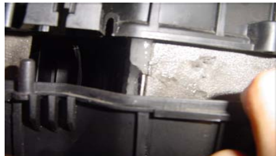
Fig. 6. Icing example of evaporator inner duct.
