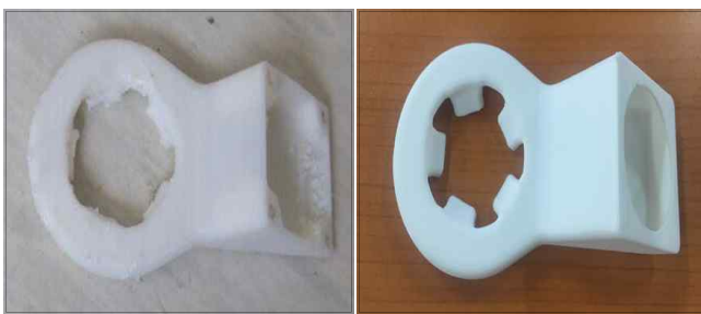
Fig. 14 3D Print comparison in one direction and 360° direction
