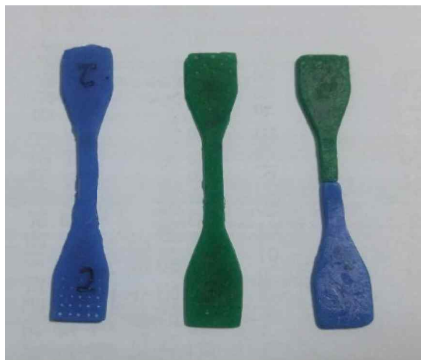
Fig. 12 Printed tensile specimen (left: blue, middle: green/right: green+blue)
