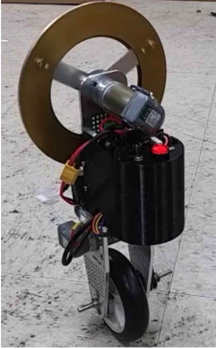
Fig. 3 Proposed single-wheeled robot
