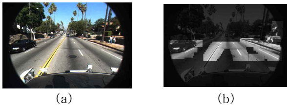
Fig. 1. Lane detection results using Haar-like feature based detector (a) input image, (b) result image.
