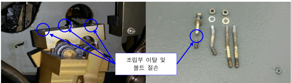
Fig. 10. The breakaway from lever support cover and The fracture of bolts
