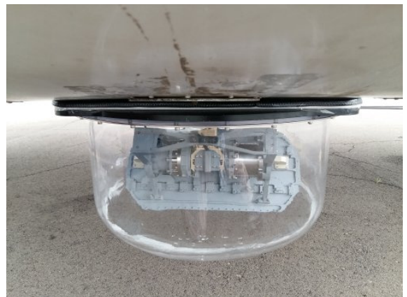
Fig. 3. The antenna and gimbal set installed to PIPER aircraft
