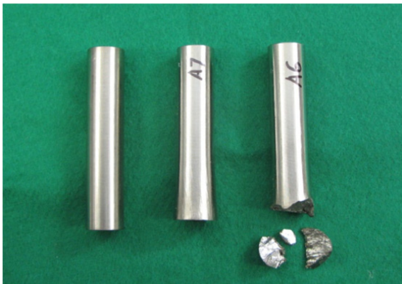
Fig. 7. Result of high velocity impact test
