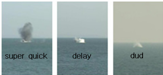
Fig. 1. Shapes of the water plumes depending on the function of the PD fuse on sea surface (captured by video camera)
