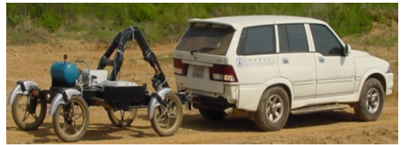
Fig. 1. 2D road profile measuring system of CPG
