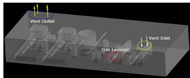
Fig. 6 Height of leakage on the 3-D modelling for FGS room
