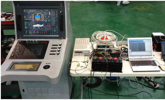
Fig. 6. Configuration of bench test for FCC redundancy
