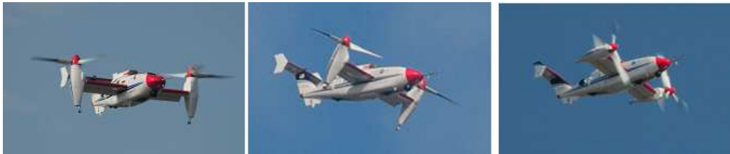
Fig. 1. Tiltrotor UAV flight configuration (rotary wing, conversion, fixed wing)
