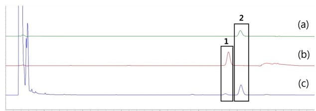
Fig. 2. HPLC Chromatograms of compounds 1, 2 and Ephedra intermedia . (a) (-)-ephedrine, (b) (+)-pseudoephedrine and (c) Ephedra intermedia .
