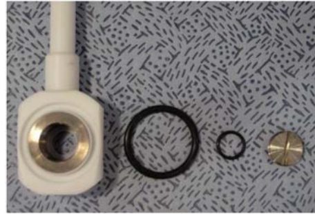
Fig. 1. Accessories of electrode holder for electrodeposition [11].
