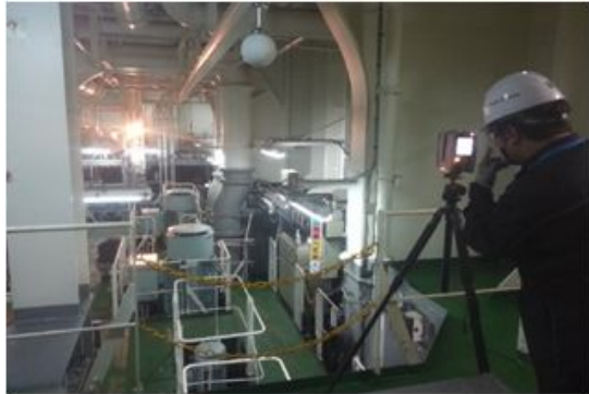
[Fig. 4] Scan Survey in Engine Room
