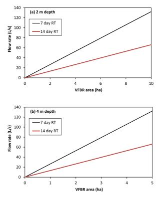
**Fig. 4.** Flow capacity for VFBRs as a function of surface area, assuming residence time (RT) of 7 days and 14 days. A (a) 2 m and (b) 4 m depth of the active vertical flow bed and an active pore volume of 40% were assumed. Note the difference in scale for the VFBR area between (a) and (b).
