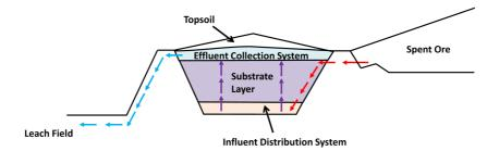
Fig. 2. Schematic cross section of a VFBR.
