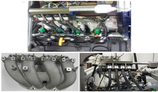
Fig. 2. Gas injection system installation on the intake manifold
