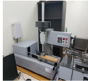
Fig. 4. 동적하중시험(Caster wheel test).
