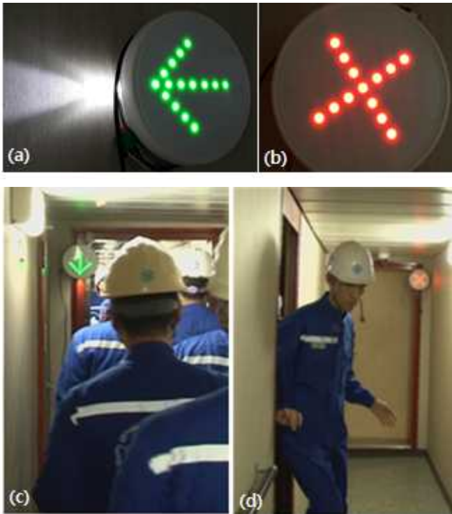
Fig. 7 (a) and (b) are photos of situation-aware escape guiding device. (c) and (d) are photo of escape experiment at T/S SAEYUDAL with the escape guiding system.
