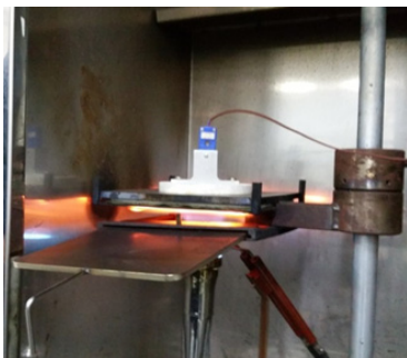
Figure 2. KS K ISO 9151 test apparatus (dimensions in millimeters).
