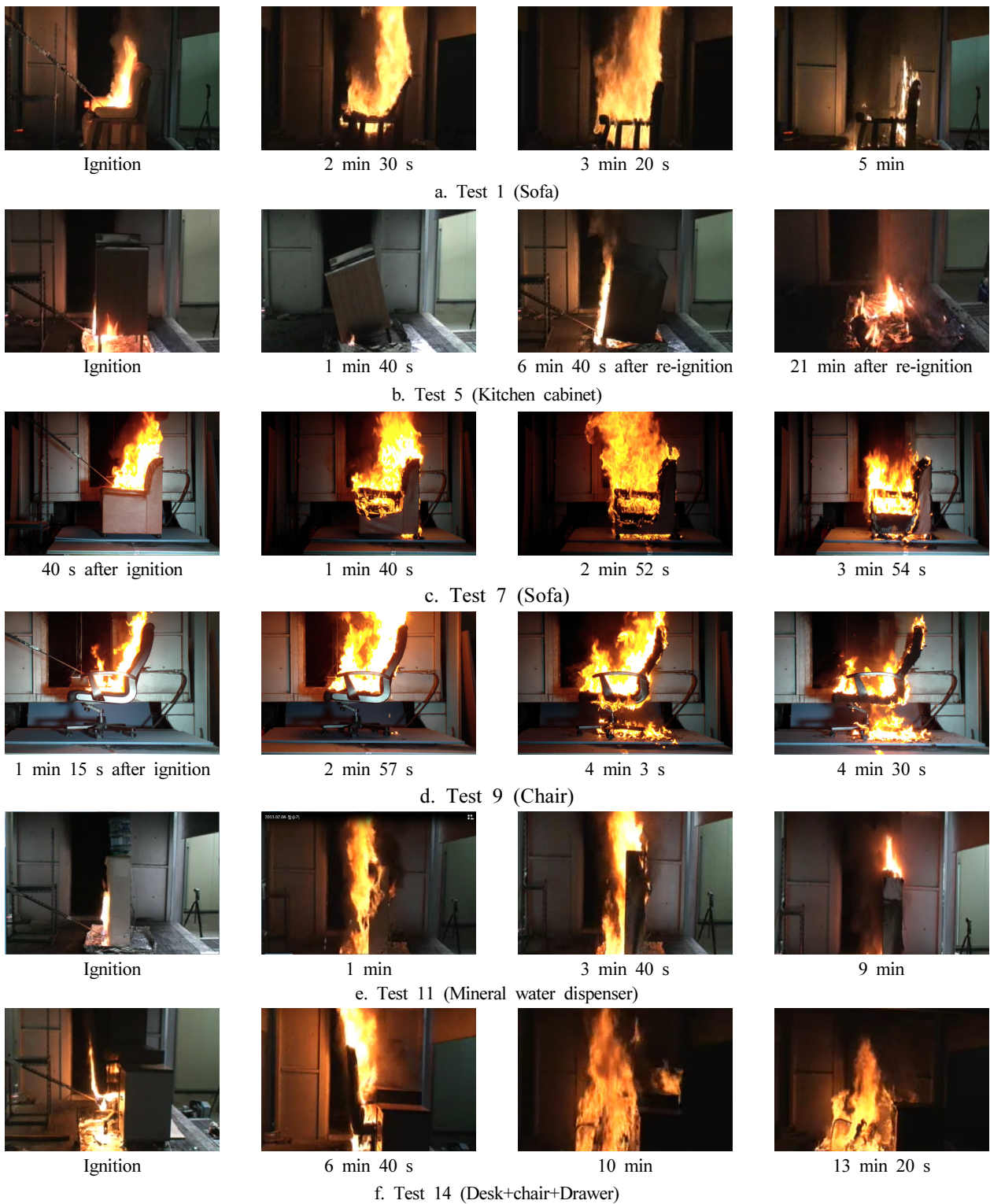
Figure 4. Burning behaviors of major combustible materials over time.
