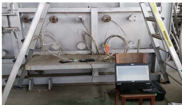
(C) Junction Thermocouple Wires to Data Pack
