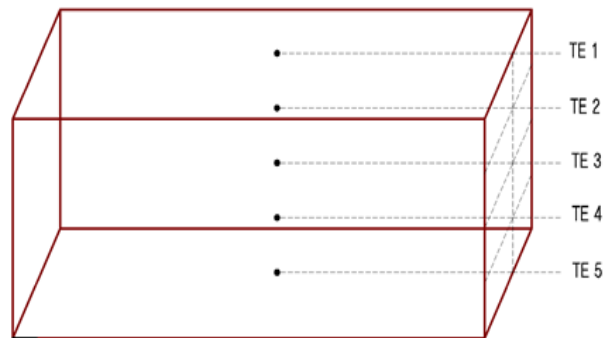
(B) Mounting Position of Thermocouples
