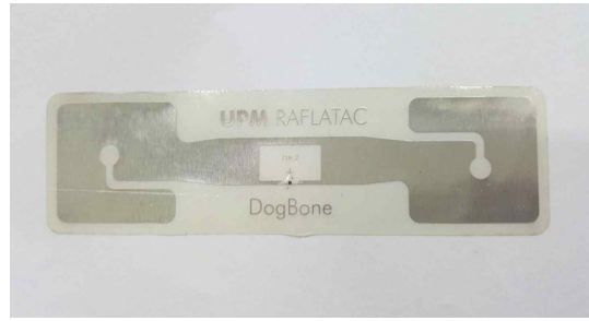
Fig. 1. The RFID tag used in the experiment.
