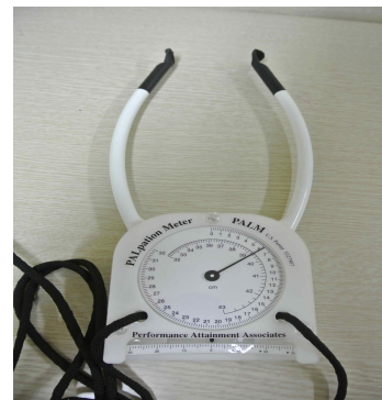
Figure 2. Palpation meter used to measure the pelvic angles in the sagittal and coronal planes.
