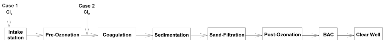
Fig. 1. Process train of drinking water treatment process in the downstream of Nakdong river.
