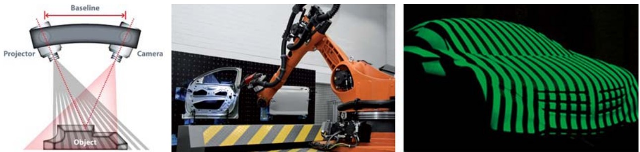
Fig. 4 Application of fringe projection in mechanical industries
