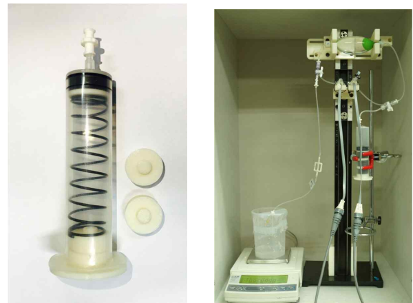
(a) Spring assist device (b) Drug infuser setup
