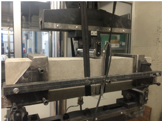
Fig. 9 Three-point bend test of prismatic notched specimens with weight compensation.
